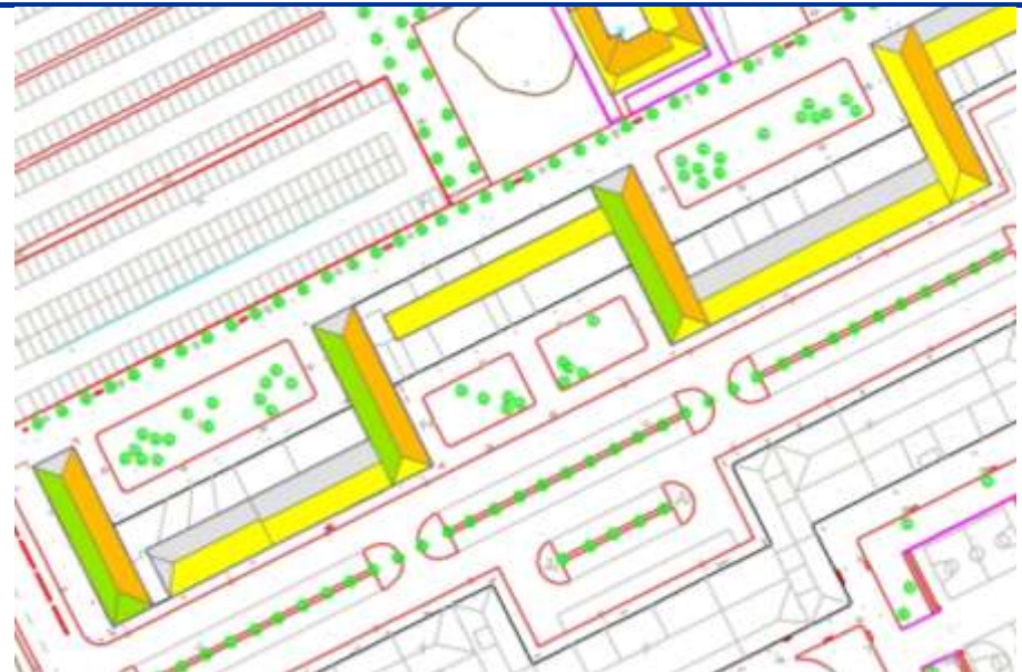
Fig. 3. Map sample applying mean radiation values for each roof part and considering filters to identify roof parts which are actually suitable for installing Solar panels. Some of these filters are surface available, building protection and structural conditions.
